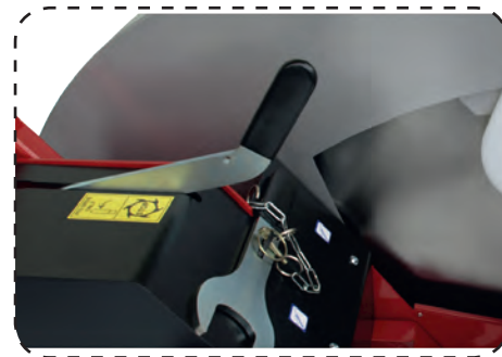
Emergency stop lever at PTO
