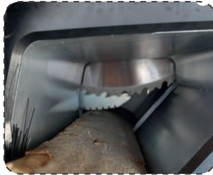
Log grip system locks the wood while sawing.
