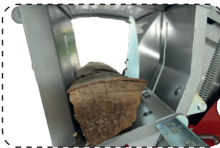
Log grip system locks the wood while sawing
