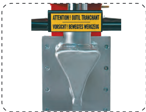
Ergonomic knife in wedge shape for splitting easily. Inclined returns to maintain the wood.
