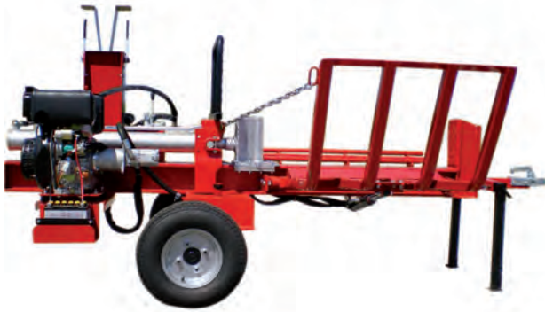
HES16-1100 Autonomous model on axle with fork (option) and hitch. Road not homologated.
