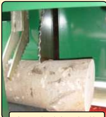
Automation timber grip with 'No grip - No Saw'
