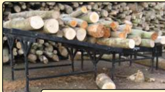
Hydraulic Timber deck Options:- 2 metre x 2 chain with 4 metre storage ramp. 3 chain deck with singulator 2 - 4 or 6 metres.
