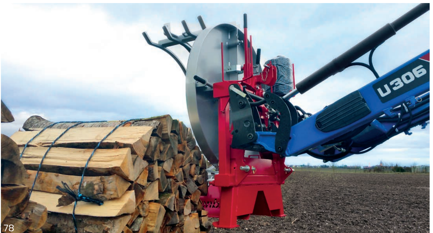
Bundler with polyester strips mechanical pivoting on 3-points hitch + euro linkage for front loader
