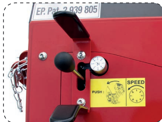
Valve and speed regulation for log carriage
