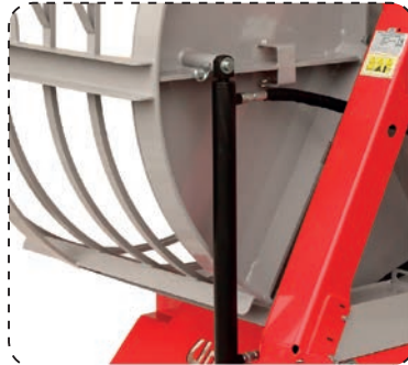
Hydraulic pivoting (left or right)
