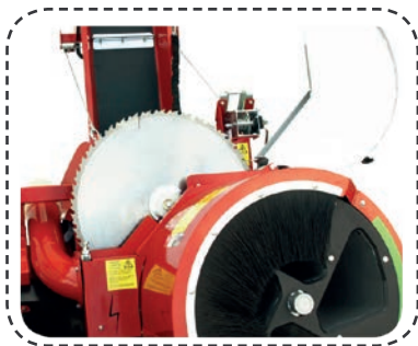
The blade is fully protected for safety but easily accessible for change
