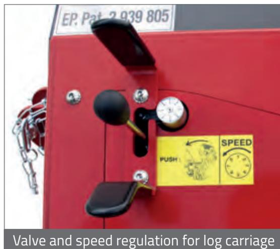
Valve and speed regulation for log carriage
