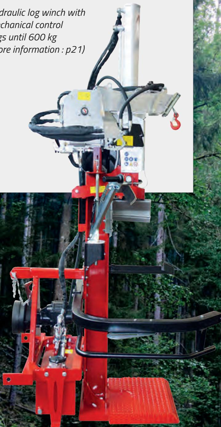
Log winch with winding limit switch
