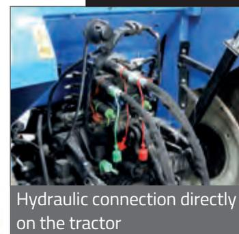
Hydraulic connection directly on the tractor
