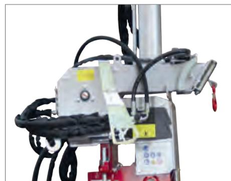
Hydraulic log winch with mechanical control system and switch at the end of winding
